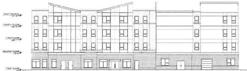
1 BLDG. C WEST ELEVATION
